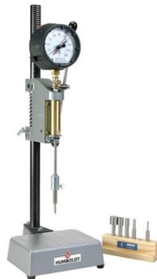
Figure 4.5. Apparatus of Penetration Resistance Test
